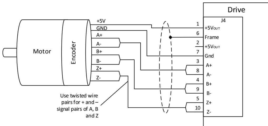
Figure 16: Differential encoder connection to the drive
