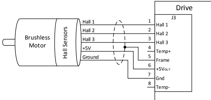
Figure 14: Hall sensor connection to the drive
