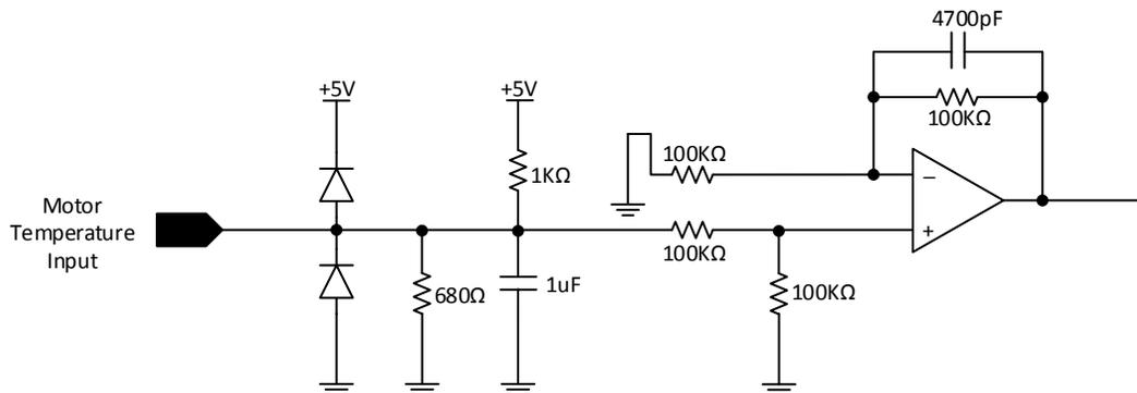
Figure 20: Temperature sensor signal input circuit
