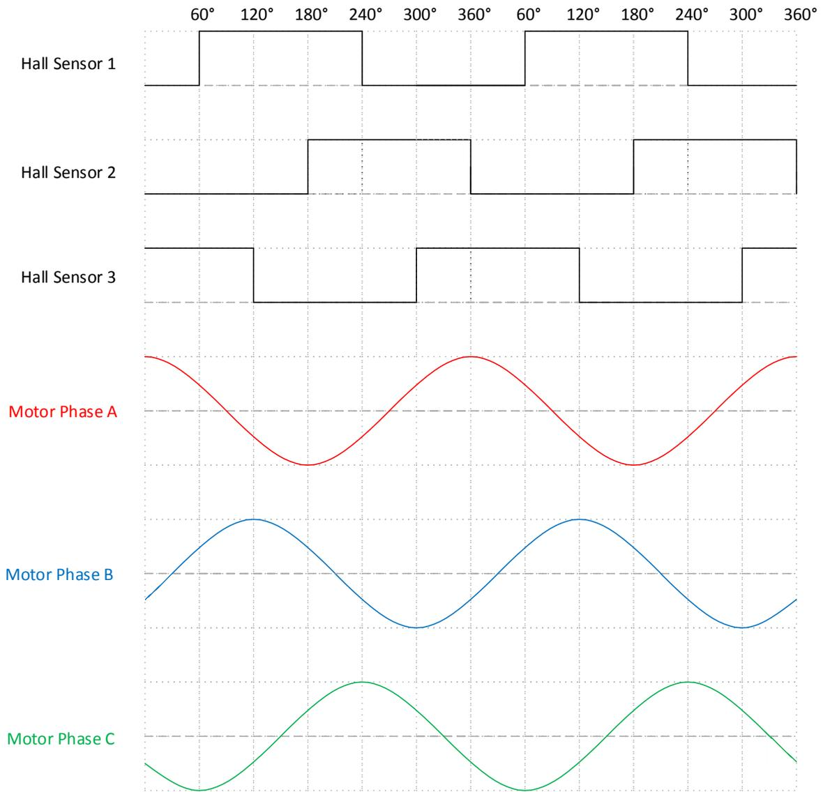
**Figure 3: Sinusoidal commutation with Hall sensor feedback**
