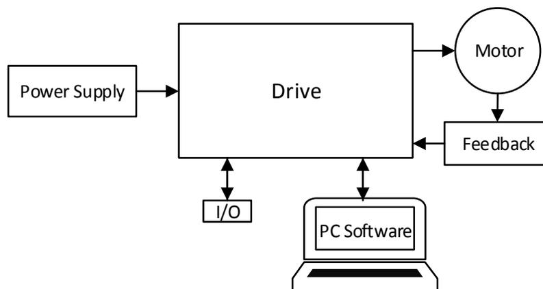
**Figure 1: Overall drive system block diagram**
