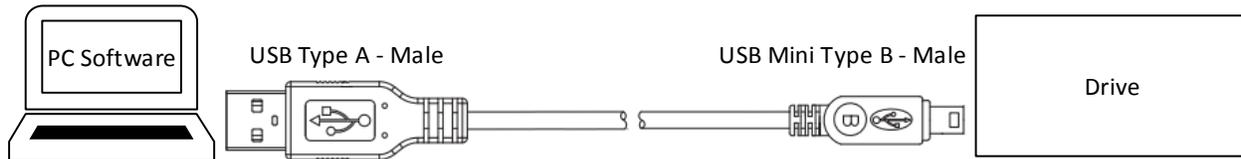
Figure 27: USB cable connection between computer and drive
