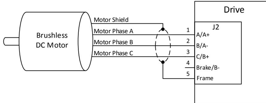
Figure 11: Brushless DC motor connection to the drive
