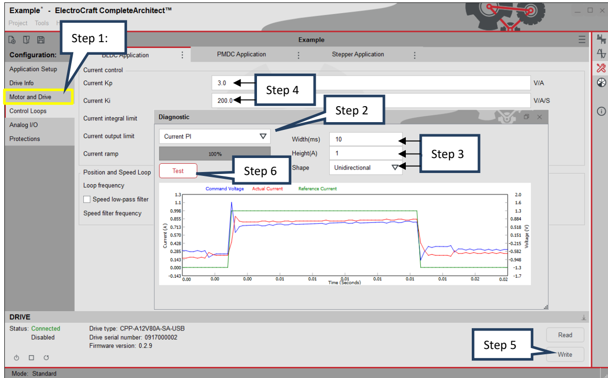
Figure 56: Critically-damped Current Control Loop
