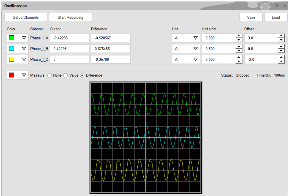
Figure 51: Sinusoidal Motor Phase Currents Plot
