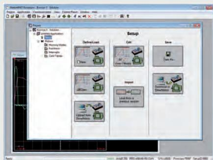
Motion profiles can be programmed online or offline. Operators can
