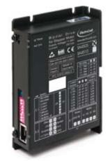
is protected against over-current and overtemperature and incorporates the state of the art dual full bridge MOSFET driver for maximum efficiency. Connectivity is tool-free with RJ45-CAT5 plugs for the control inputs and push-type terminals for power. The optically isolated control circuit can be powered with the internal 5V supply on the drive for TTL step and direction compatibility or supply an auxiliary voltage supply for up to 24V logic step and direction.
